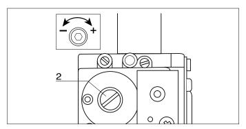
If the value measured corresponds to the value given in the table, adjustment is complete, otherwise start the setting procedure again.
