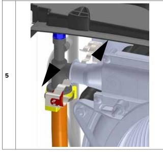
Disconnect the plastic pipes from the manual air vent.
