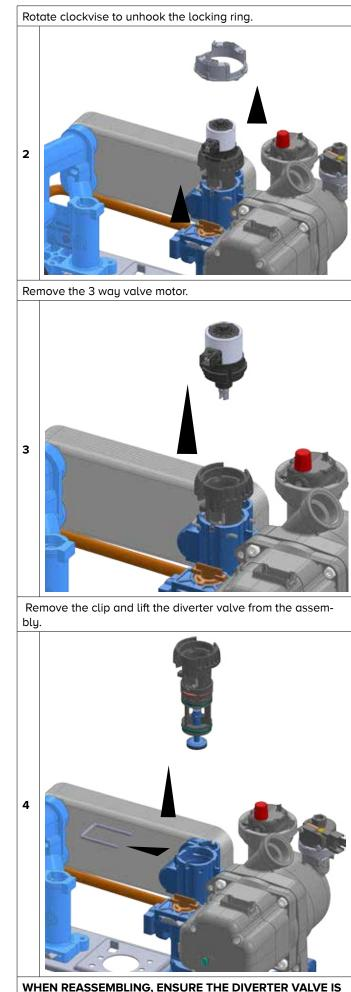
WHEN REASSEMBLING, ENSURE THE DIVERTER VALVE IS ALIGNED CORRECTLY.
