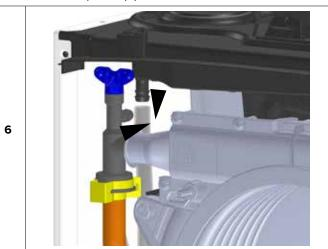
Disconnect the heating flow pipe
