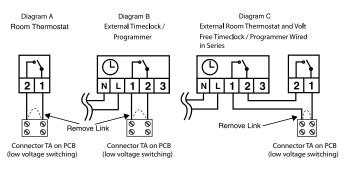
Timeclock and Room Thermostat low voltage compatible
