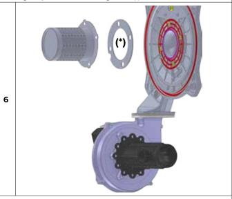
Verify and replace the other gaskets if they are damaged or showing signs of deterioration
