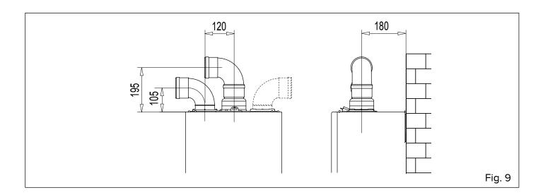
For coaxial systems, the maximum development value, mentioned in the table below also takes into account an elbow. For twin flue systems the maximum development value, mentioned in the table includes the exhaust gas/air intake terminal.
