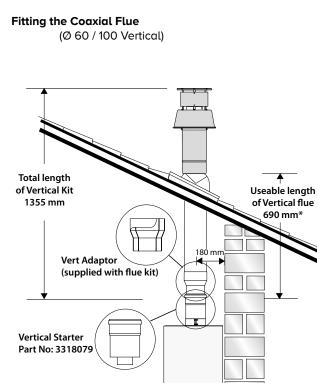
\*This length will vary according to the type of flashing installed
