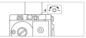
If the value measured corresponds to the value given in the table, max adjustment is complete, otherwise start the setting procedure again.
